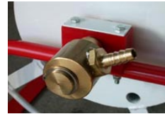
Standard Brass Supply Swivel 3/8", 1/2" ( 1000psi) 3/4",1" (750psi)
